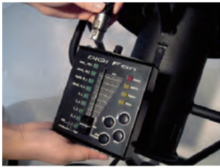
Multi functional control box for Manual, DMX and Program setting.
