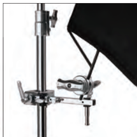
KS-010 Offset Arm 215mm (8.4") W 540g 19oz Steel made offset arm with a two hex adapters, one on the end of the arm and another at a right angle to it for mounting flexibility. The other side of the arm features two opposing baby 5/8" pins for mounting light fixtures or any other baby accessory with a baby receiver.
