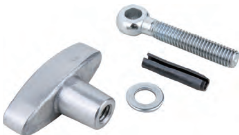
KS-192 Eye Bolt w/ Aluminum Knob W 180g / 6.35oz Chromed plated 1/2"-12 eye bolt with aluminum casting knob can be a replacement of the eye bolt with wing nut which is equipped on the coupler by means of removing the spring pin.
