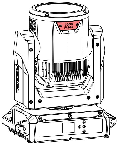
Gently screw the new Logo Plate into place, making sure it is flush and straight. Do not overtighten to prevent damage to the badge or the fixture.
